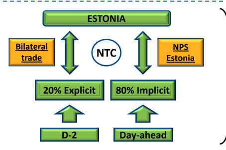
The problem of scarce cross border capacity between Estonia and Latvia is aggravated by the fact that only 80% of net transfer capacity (NTC) is allocated for trades which participate at the Nord Pool Spot (NPS).
